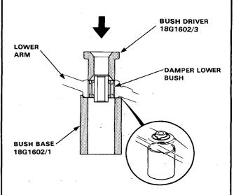
2. Drive the rear damper lower bushing from the direction indicated.
