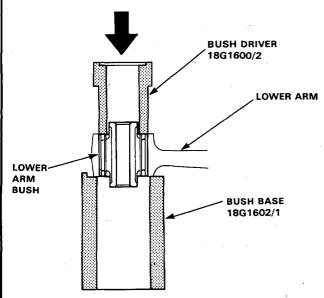
2. Drive the rear lower arm bushings from the direction indicated.
