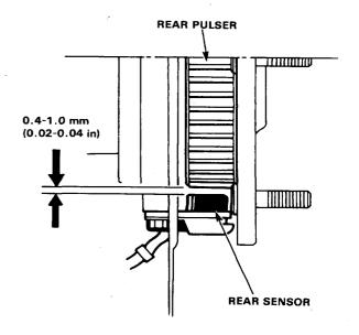
Measure the air gap between the sensor and pulser all the way around while rotating the hab bearing unit by hand.
