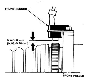
Measure air gap between the sensor and pulser all the way around while rotating the driveshaft by hand.
